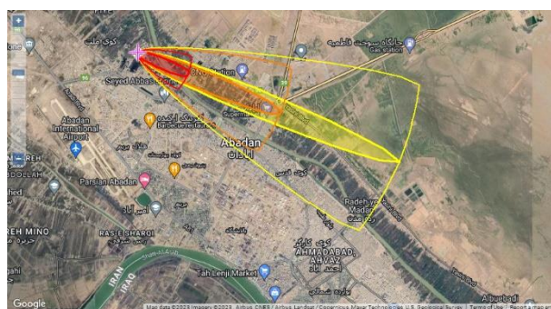
Figure 4. Radius of diffusion and chlorine gas concentration of 1 tonne
