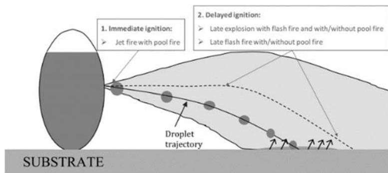
Figure 2. Continuous release of flammable material with rainout [4]
