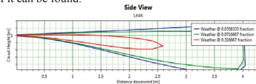
**Figure 11.** Leakage with a diameter of 25 mm from the ethanol tank from the side view
