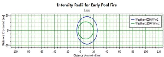
**Figure 12.** Pool fire radiation at the initial moment of leakage to a diameter of 25 mm from the ethanol tank at the initial moment
