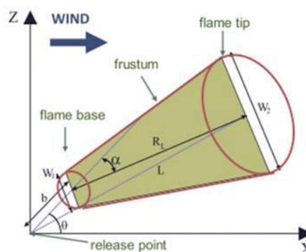
**Figure 5.** Geometry for pool fire (tilted cylinder) and jet fire (cone) [4]
