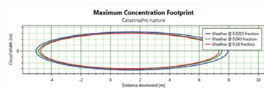
**Figure 19.** Ethanol Tank catastrophic rupture and release clouds from above view in winter
