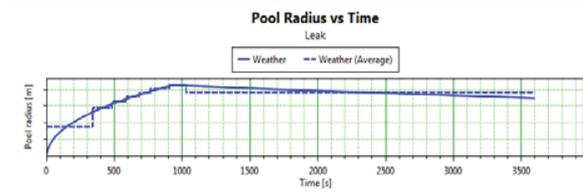
**Figure 9.** Ethanol leak with a diameter of 100 mm from the tank and the creation of a pool fire appropriate to the time in summer
