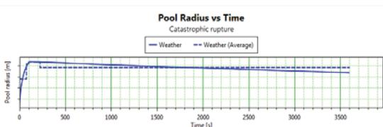
**Figure 21.** Rupture of ethanol tank and create pool fire in terms of time in winter
