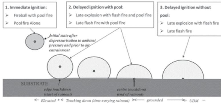
Figure 3. Instantaneous release of flammable material with rainout [4]
