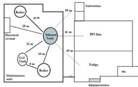
**Figure 8.** Schematic diagram of ethanol tank from other equipment
