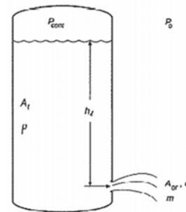
Figure 4. Symbolic form of draining liquid from a tank
