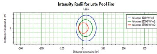
**Figure 15.** Pool fire radiation from a leak with a diameter of 25 mm from the ethanol tank
