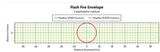
**Figure 20.** Rupture of ethanol tank and cause Flash fire in winter
