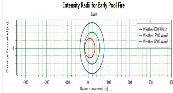
**Figure 6.** Radiation caused by ethanol leakage to a diameter of 100 mm from the tank and the formation of a pool fire without delay in summer
