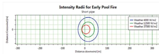
**Fig. 16.** Radiation from a 3-inch-diameter ethanol leak from a Short pipe tank and the creation of a pool fire in summer
