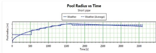
**Figure 18.** Ethanol leakage 3-inch-diameter from the Short pipe tank and create a pool fire appropriate to the time in summer
