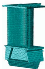
Figure 4. Turbine blade 3-d finite element model [25]
