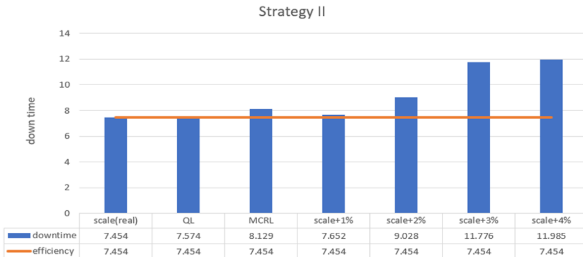
Figure 7. System downtime of different approaches under minor changes in the Weibull scale parameters for Strategy II
