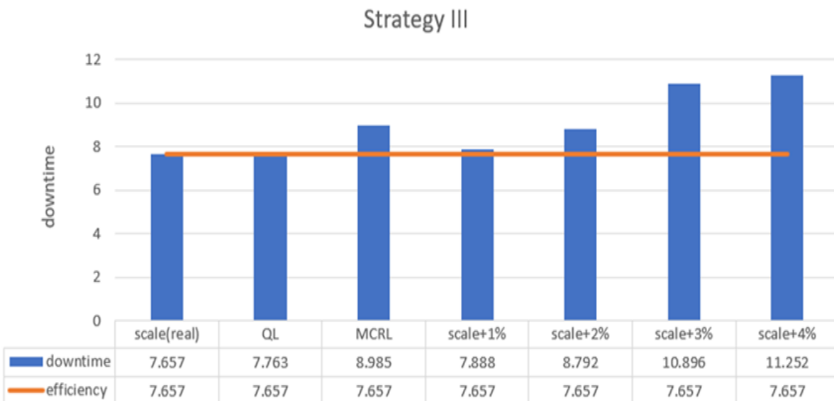
Figure 8. System downtime of different approaches under minor changes in the Weibull scale parameters for Strategy III
