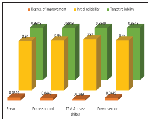
Figure 7. Comparison of allocated reliabilities to critical subsystems for a duration of 5000 hours of (of) work
